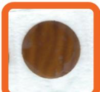
Fig. 1 Film indicator for sulfur dioxide content
