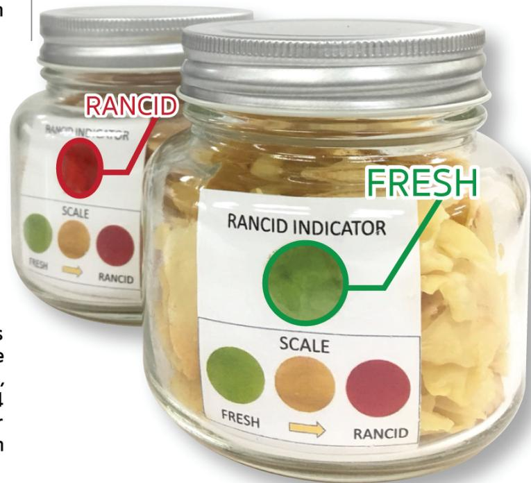
Fig. 3 Film indicator color changing comparison after stored in Durian chip container with different PV.
